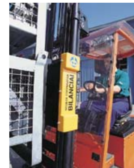
Detail showing the side cover protecting the flexures and the load cells.
