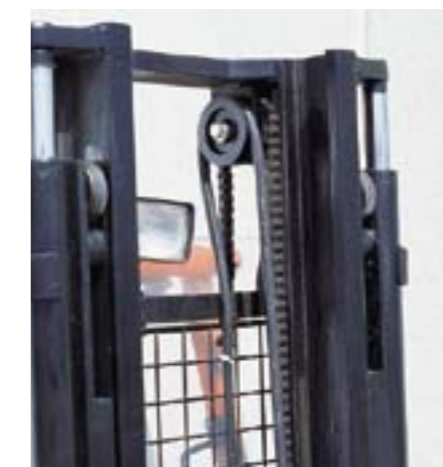
Connection of terminal to the truck scale with pulley system; recommended for two/three mast extensions.
