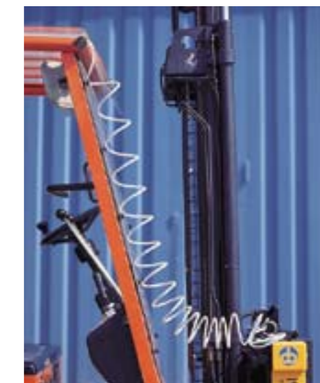
Connection of the terminal to the truck scale via coiled cable; recommended for masts with one/two extensions.
