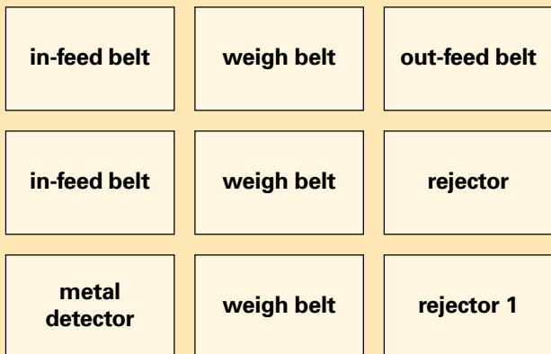
→ packs are rejected when metal is detected or the weight is wrong.
